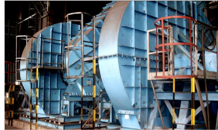
Radial ventilator for power plant
