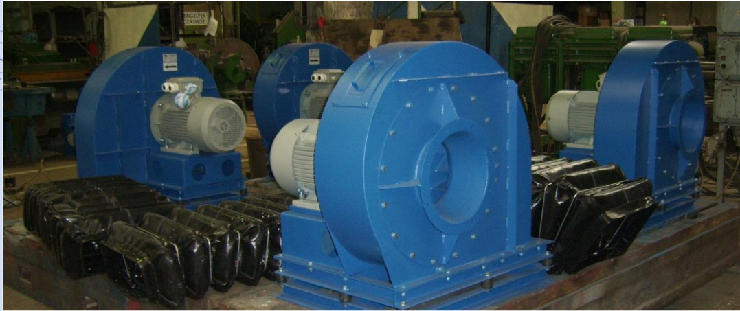
MDSk-56 radial ventilators with their compensator
