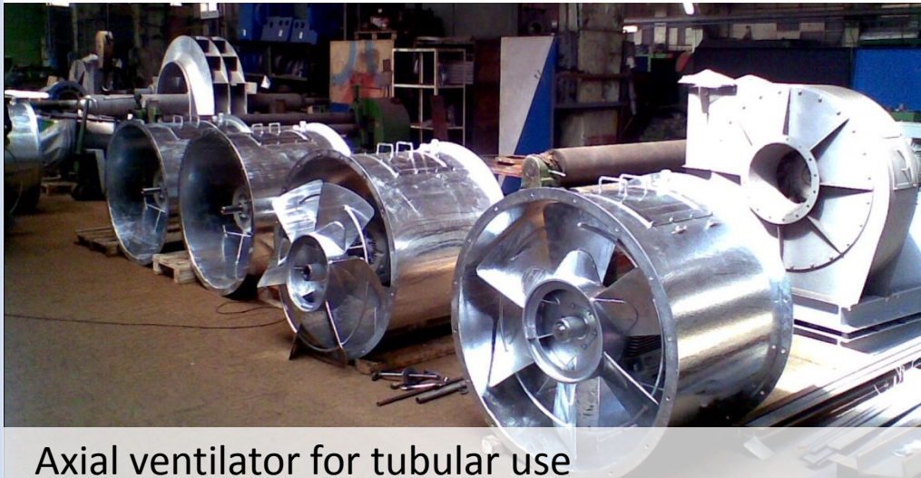
Impeller with adjustable blade angle
